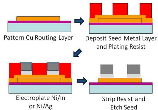
**Figure 5, Diagram of process used to form routing metal and 10  $\mu\text{m}$  pitch Ni/In or Ni/Ag microbumps.**
