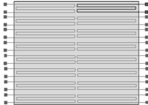
**Figure 4, Schematic diagram of the testing structure in plan view showing the layout of the individual test channels. Each die contains 128 channels on each side and each test channel contains 1280 microbumps connected in series.**
