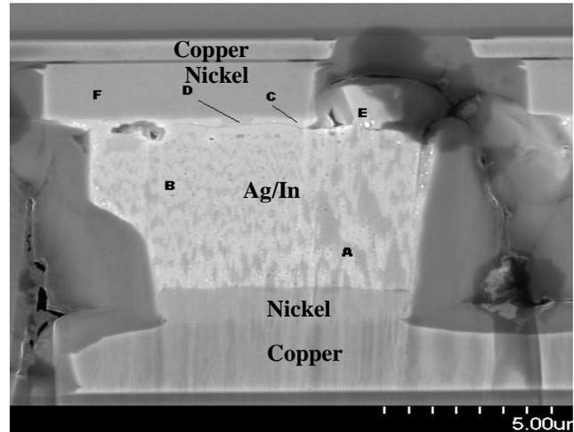
**Figure 6, Bond cross-section showing EDS locations**
