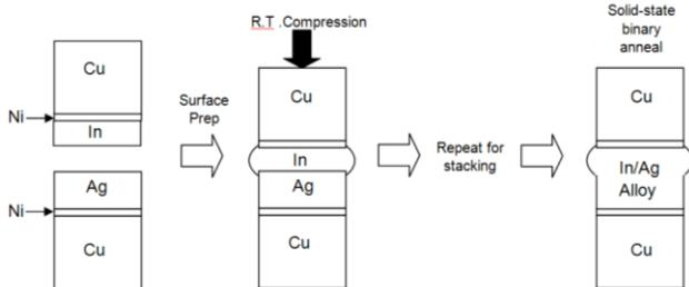
**Figure 3, Proposed interconnect design and process.**
