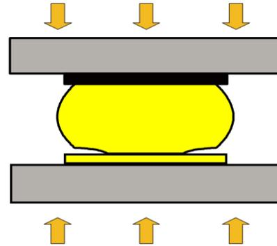
**Figure 2, Thermocompression bonding**
