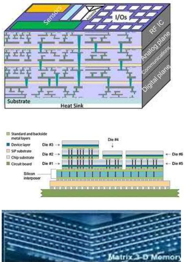
Figure 1, Examples of 2.5 and 3D structures
